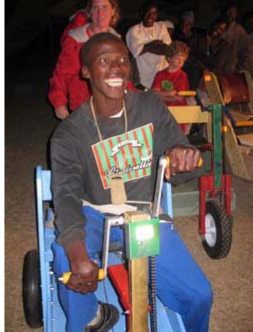
PET wheelchairs are designed for the unforgiving African bush. This is a "crank" chair operated by the patient himself.
